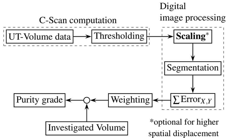
Figure 9: SEP1927 workflow using a ultrasonic volume scan
