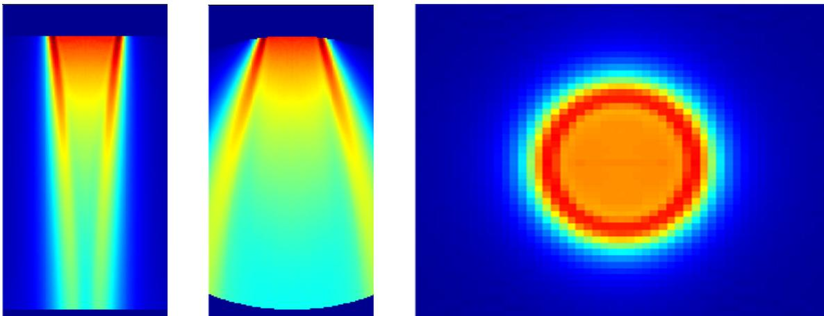
Figure 2: Directivity pattern of the transducer stated by ASTM E588 x-zone (top left), y-zone (bottom left) and focal point (right) in material
