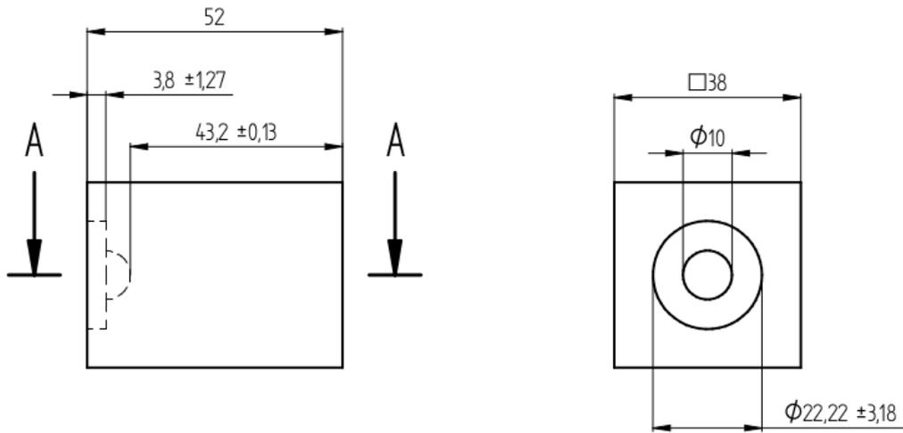
Figure 6: ASTM E588 reference block
