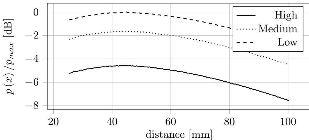
Figure 5: ASTM E588 reference levels for gate counter alignment over distance
