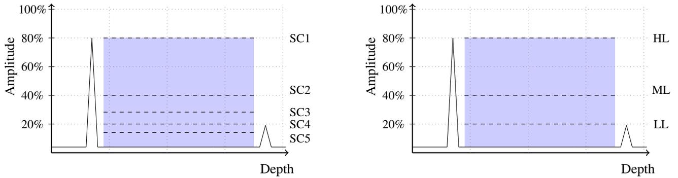
Figure 8: ROI comparison SEP 1927 (left) and ASTM E588 (right)
