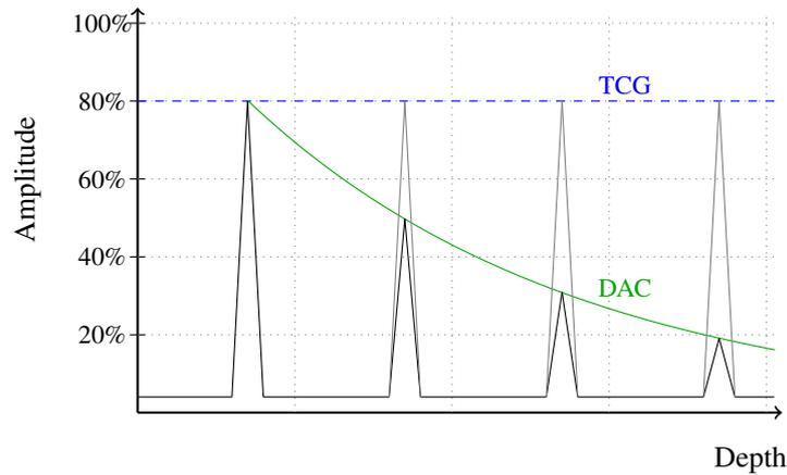
Figure 4: Distance amplitude correction (DAC) and corresponding time gain correction (TGC)
