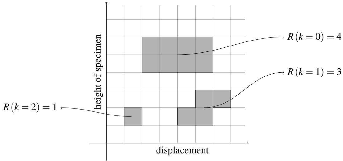
Figure 10: Example of a binary C-Scan interpretation by SEP1927
