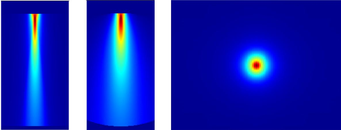
Figure 1: Directivity pattern of the transducer stated by SEP1927 x-zone (top left), y-zone (bottom left) and focal point (right) in material
