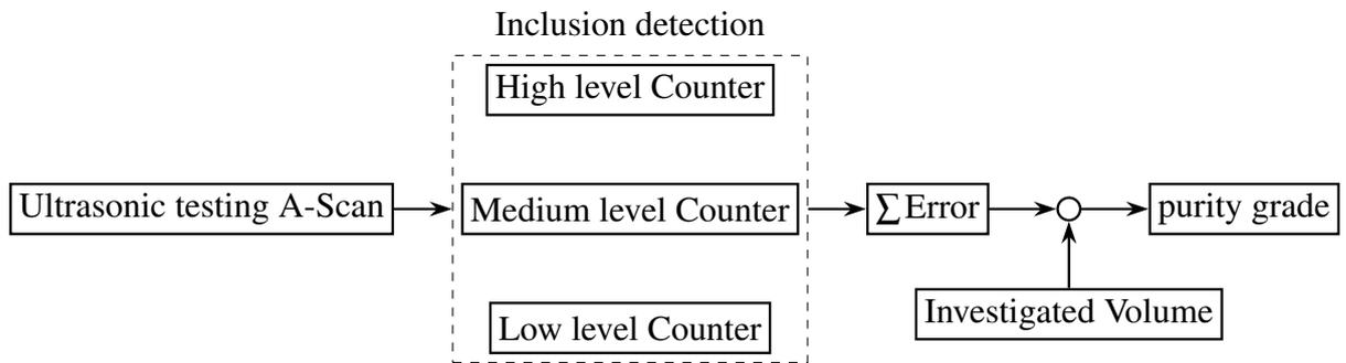
Figure 11: ASTM E588 workflow using an ultrasonic gate counter
